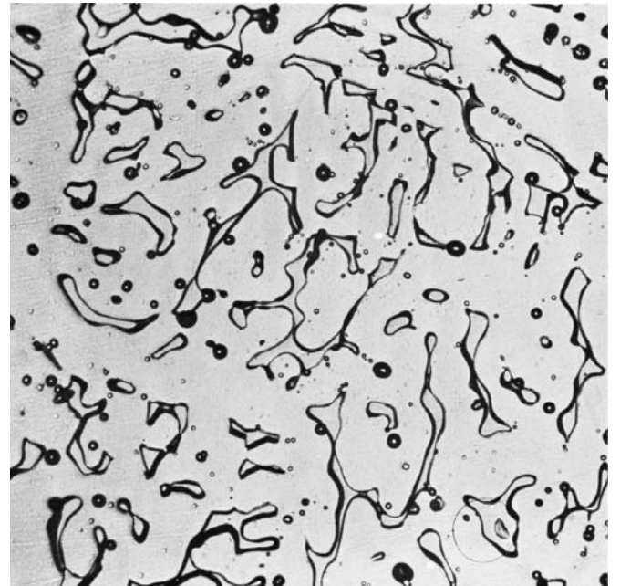
FIG. 4 Isolated Ferrite Pools (250x) (Observed in Castings and Welds. Steps Between Austenite Matrix and Ferrite Pools)
